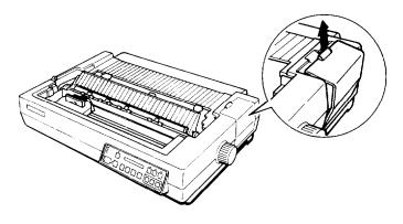
3. Using a cross-head screwdriver, remove the three retaining screws located deep inside of the slots at the front of the printer.
